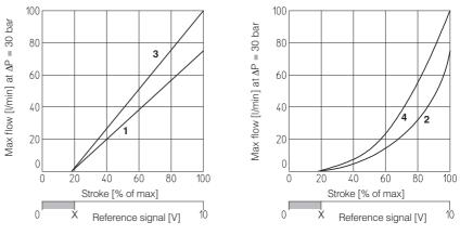
X = Threshold for bias activation depending to the valve type and amplifier type
