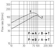
Valve pressure drop  $\Delta p$  [bar]
