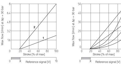
$\mathbf{X}$  = Threshold for bias activation depending to the valve type and amplifier type
